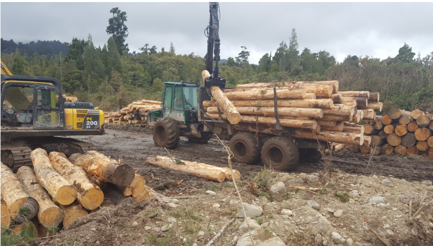
Purpose built log forwarder, can cart on cutover or tracks to load out areas
