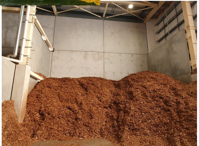
Chip material ready for burning – mix of chipped branches, pine cones & needles
